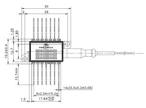
Dimensions are in mm Fiber length  $1000 \pm 90$  mm (including optical connector)
