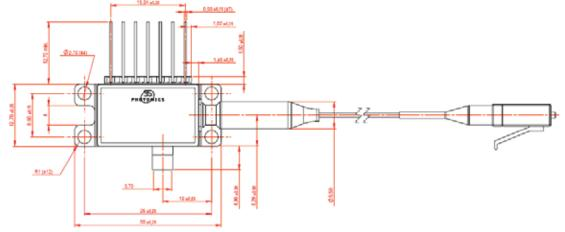
Dimensions are in mm Fiber length  $1600 \pm 100$  mm (including optical connector)
