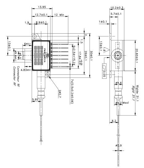
Dimensions are in mm Fiber length 1600  $\pm$  100 mm (including optical connector)
