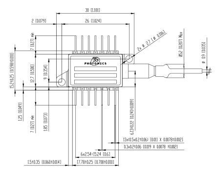
Dimensions are in mm Fiber length  $1600 \pm 100$  mm (including optical connector)
