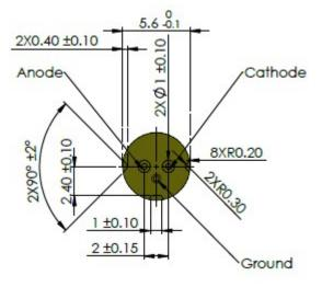
220 mW Kink-Free, FBG Stabilized, 980 nm Uncooled TO can Laser Module
