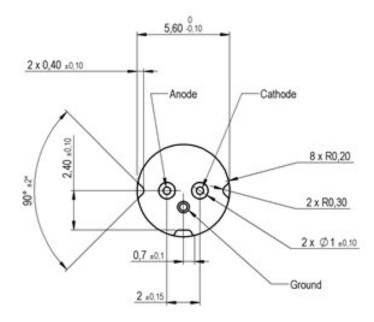
220 mW Kink-Free, FBG Stabilized, 980 nm Uncooled TO can Laser Module
