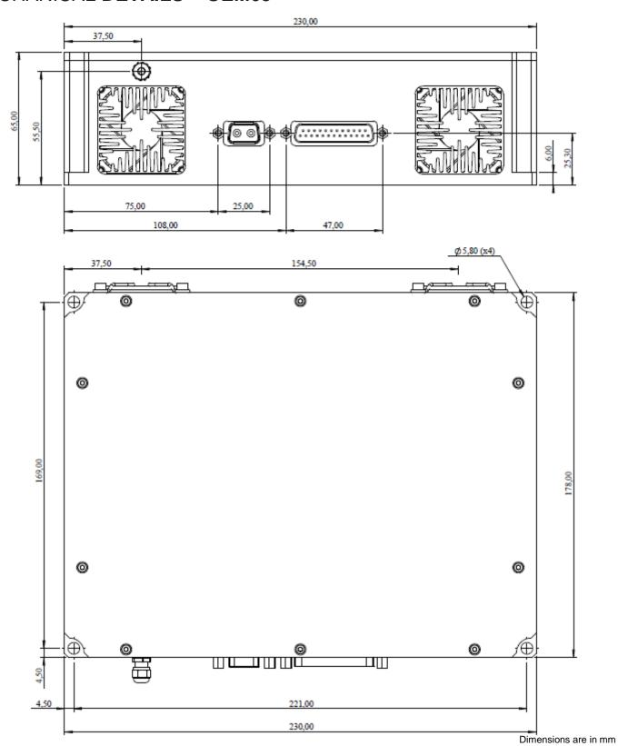
1.5 µm Pulsed High Power Fiber Laser
