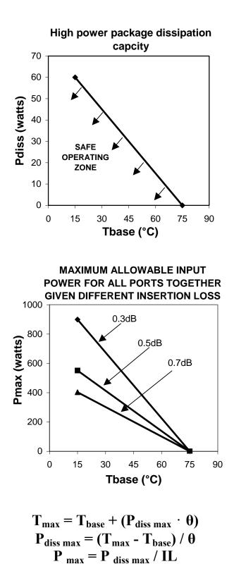
**T**<sub>max</sub>: maximum internal temperature set at 75°C **T**<sub>base</sub>: temperature at the interface of the heatsink and the package when in operation (°C) **P**<sub>diss max</sub>: maximum dissipated power (W) **IL**: insertion loss (linear scale)  $\theta$ : thermal resistance set at 1°C/W<sub>dissipated</sub>
